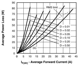
Fig. 6 - Forward Power Loss Characteristics
