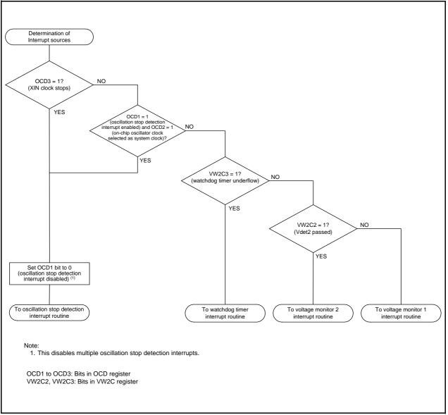
Figure 9.10 Example of Determining Interrupt Sources for Oscillation Stop Detection, Watchdog Timer, Voltage Monitor 1, or Voltage Monitor 2 Interrupt
