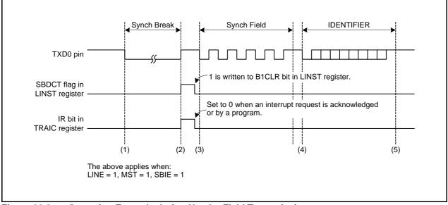
Figure 22.2 Operating Example during Header Field Transmission
