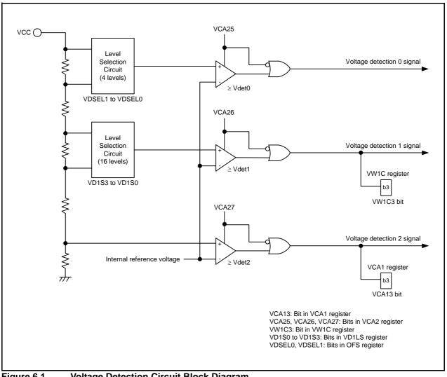
Figure 6.1 Voltage Detection Circuit Block Diagram
