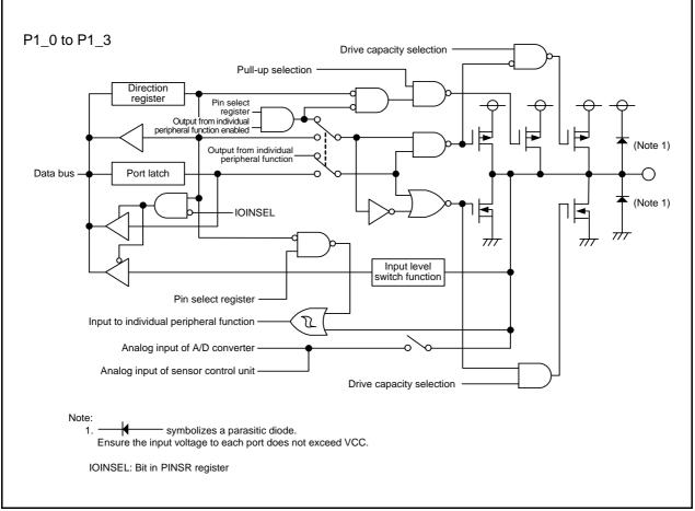
Figure 7.2Configuration of I/O Ports (2)
