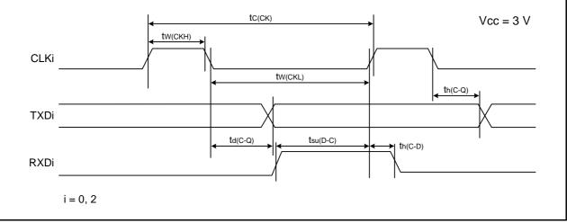
Figure 27.10 Serial Interface Timing Diagram when Vcc = 3 V
