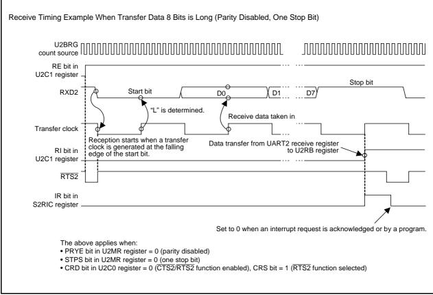
Figure 21.8 Receive Timing in UART Mode
