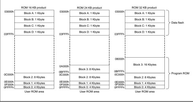
Figure 25.1 R8C/3JT Group Flash Memory Block Diagram
