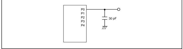
Figure 27.1 Ports P0 to P4 Timing Measurement Circuit
