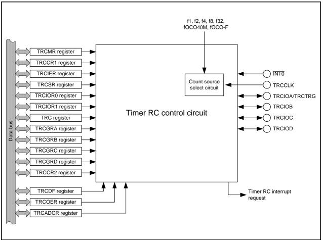
Figure 19.1 Timer RC Block Diagram
