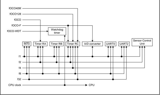
Figure 9.2 Peripheral Function Clock
