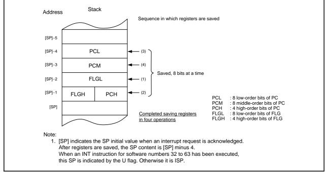
Figure 11.6 Register Saving Operation
