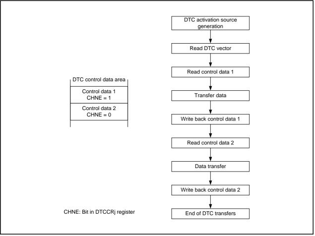
Figure 15.8 Flow of Chain Transfers
