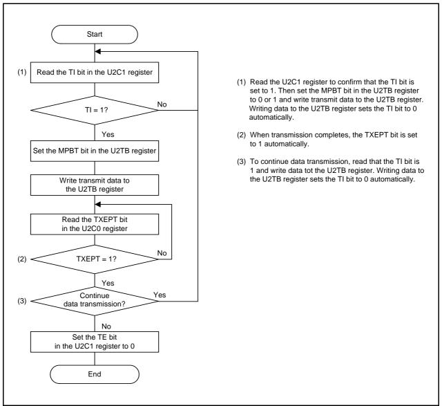
Figure 21.23 Sample Flowchart of Multiprocessor Data Transmission
