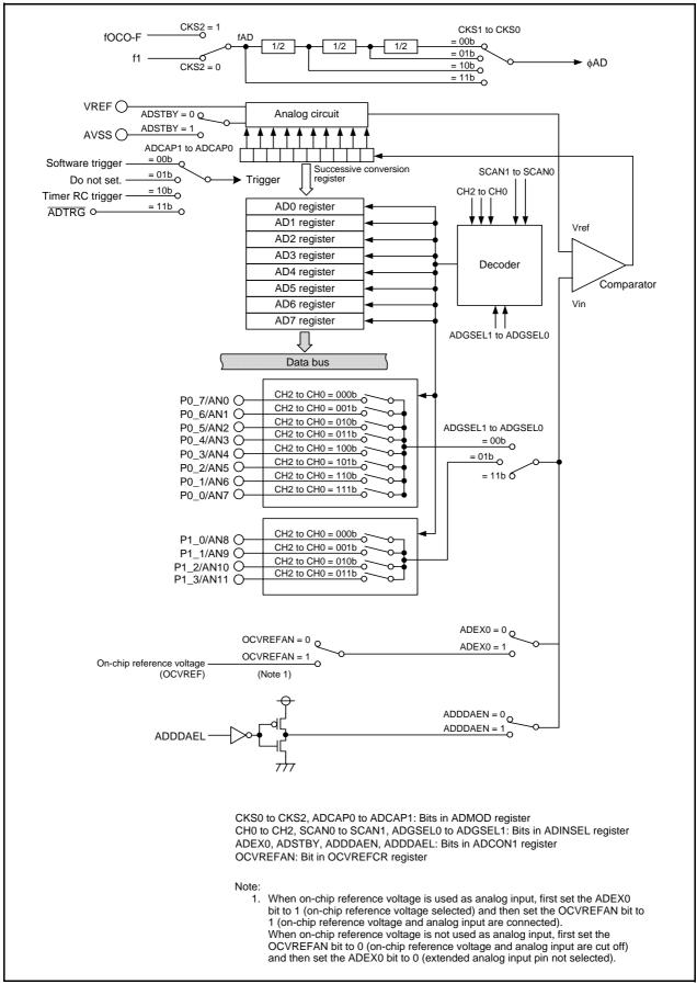
Figure 23.1 Block Diagram of A/D Converter
