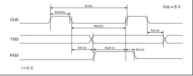
Figure 27.6 Serial Interface Timing Diagram when Vcc = 5 V
