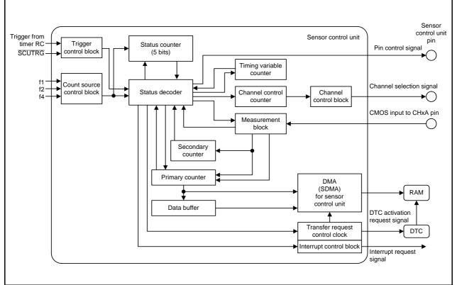
Figure 24.2 Block Diagram of Sensor Control Unit
