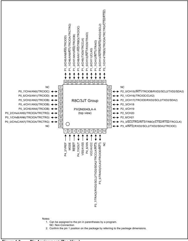
Figure 1.3 Pin Assignment (Top View)
