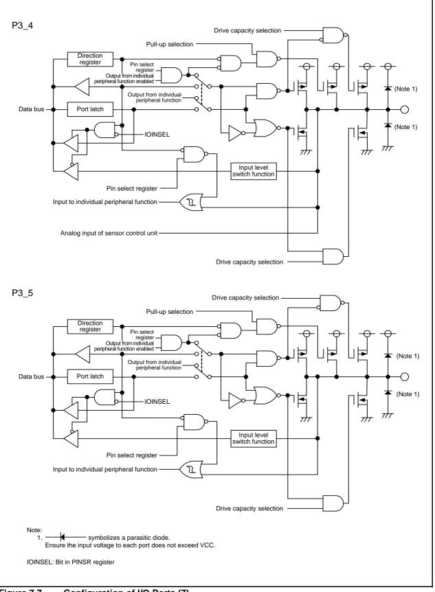
Figure 7.7 Configuration of I/O Ports (7)
