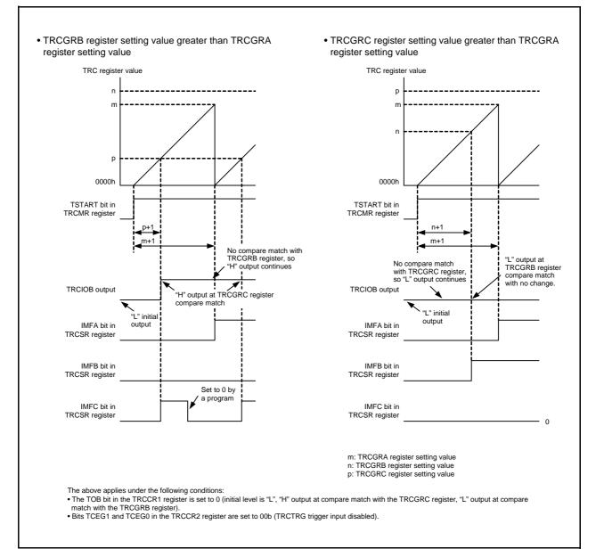
Figure 19.19 Operating Example of PWM2 Mode (Duty 0% and Duty 100%)
