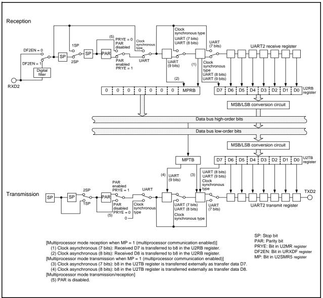
Figure 21.22 Block Diagram of Multiprocessor Communication Function
