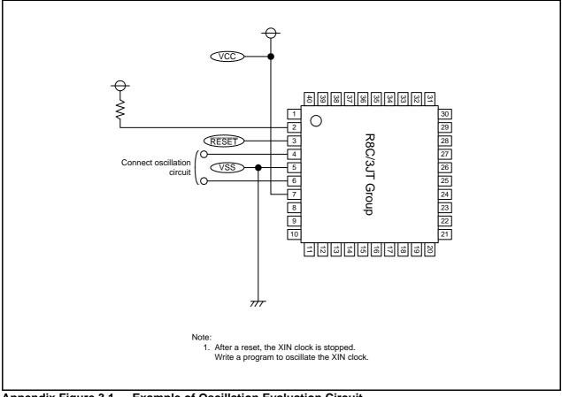
Appendix Figure 3.1 Example of Oscillation Evaluation Circuit
