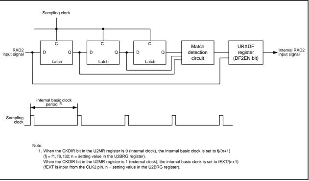
Figure 21.12 Block Diagram of RXD2 Digital Filter Circuit
