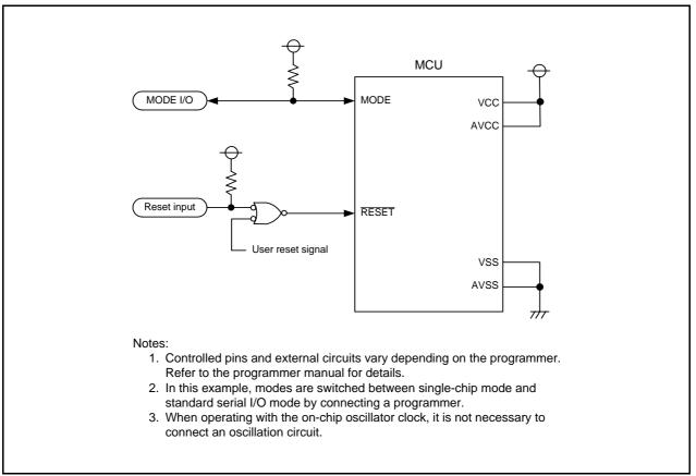
Figure 25.18 Pin Handling in Standard Serial I/O Mode 3
