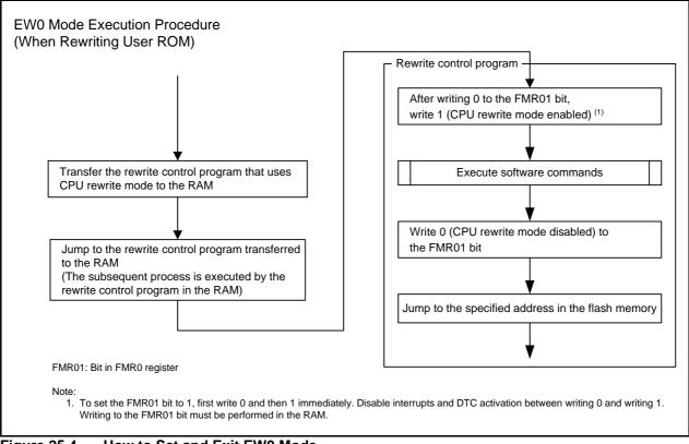
Figure 25.4 How to Set and Exit EW0 Mode
