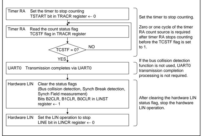
Figure 22.10 Example of Hardware LIN Communication Completion Flowchart
