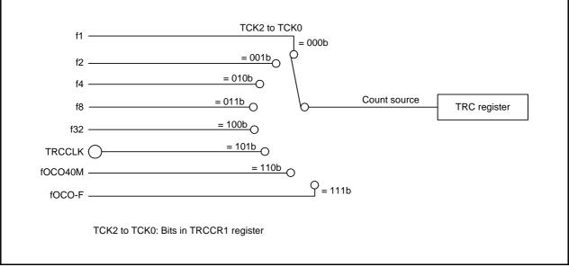
Figure 19.2 Count Source Block Diagram
