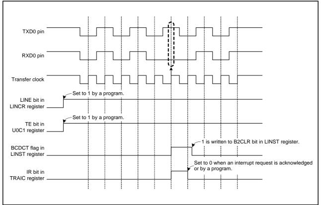
Figure 22.9 Operating Example When Bus Collision is Detected
