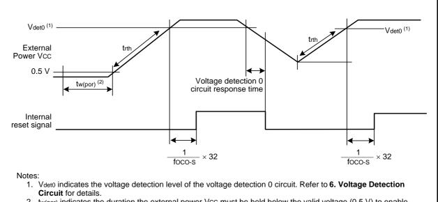
tw(por) indicates the duration the external power Vcc must be held below the valid voltage (0.5 V) to enable a power-on reset. When turning on the power after it falls with voltage monitor 0 reset disabled, maintain tw(por) for 1 ms or more.
