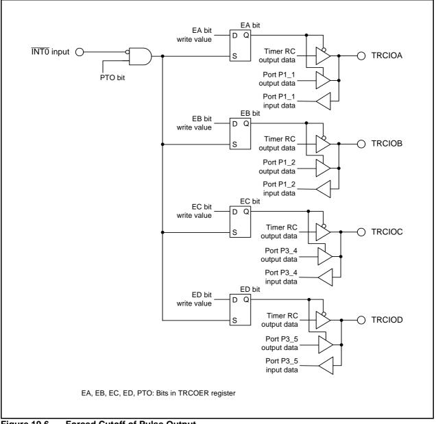
Figure 19.6 Forced Cutoff of Pulse Output
