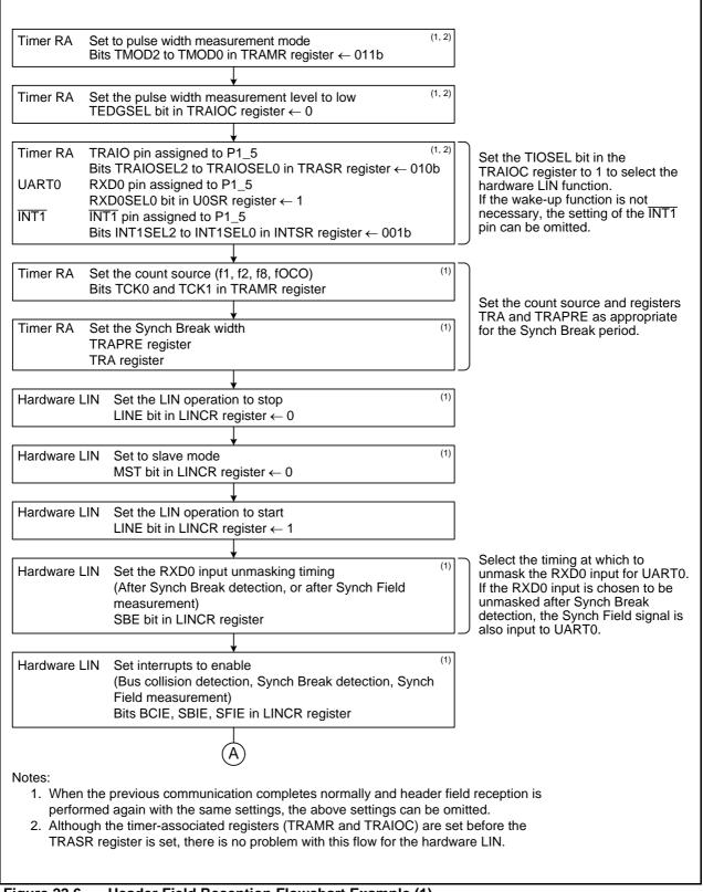
Figure 22.6 Header Field Reception Flowchart Example (1)
