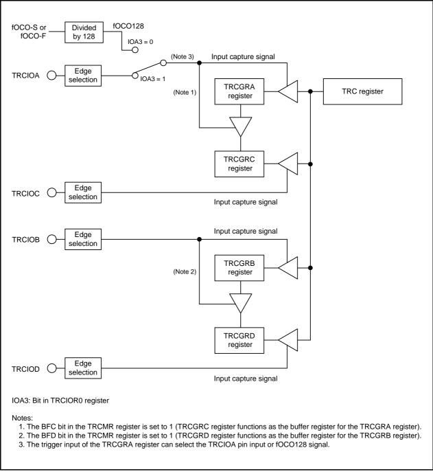
Figure 19.7 Block Diagram of Input Capture Function
