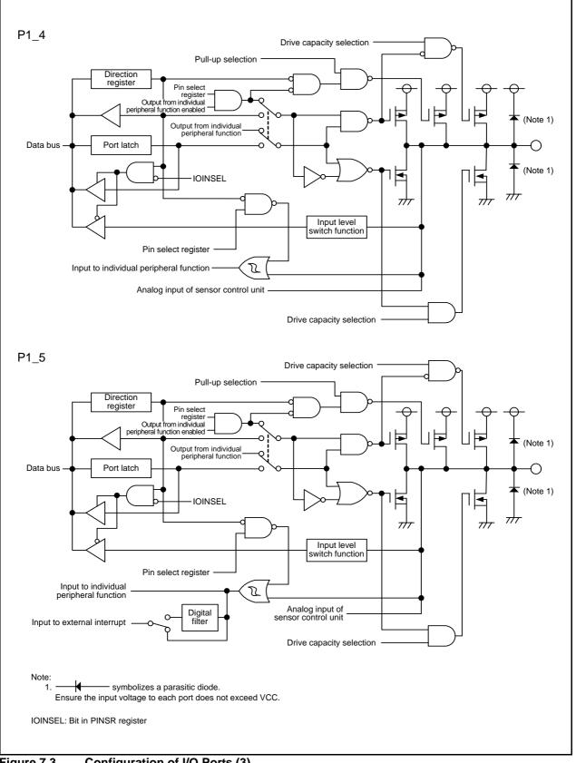
Figure 7.3 Configuration of I/O Ports (3)
