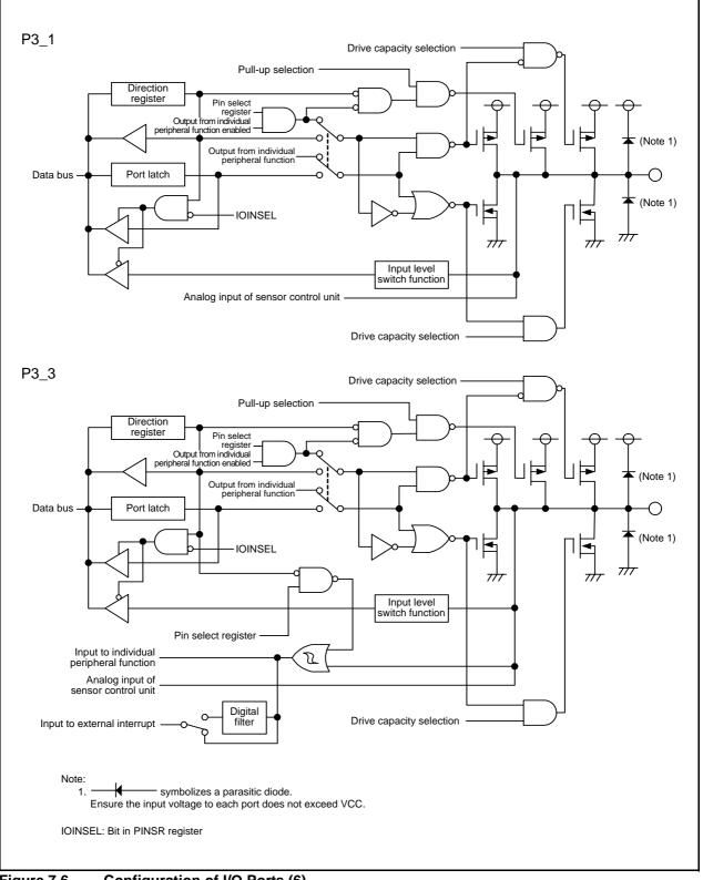
Figure 7.6 Configuration of I/O Ports (6)
