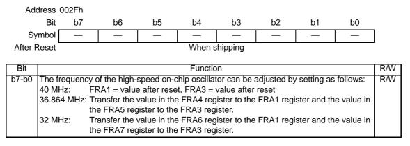
Set the PRC0 bit in the PRCR register to 1 (write enabled) before rewriting the FRA3 register. Also, rewrite the FRA3 register when the FRA00 bit in the FRA0 register is set 0 (high-speed on-chip oscillator off).
