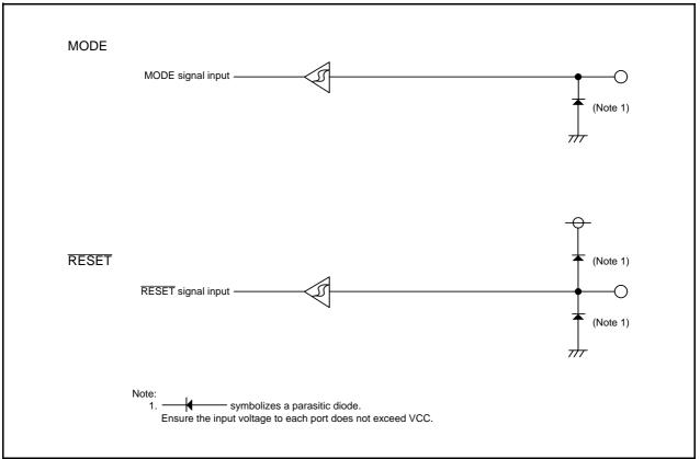
Figure 7.11 Configuration of I/O Pins
