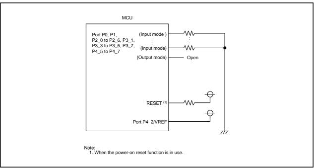
Figure 7.12 Unassigned Pin Handling
