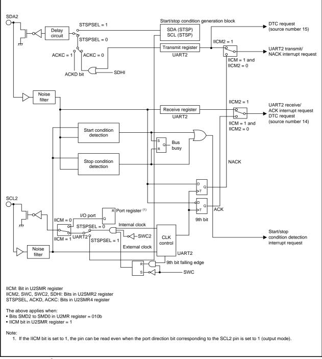
Figure 21.13 I<sup>2</sup>C Mode Block Diagram
