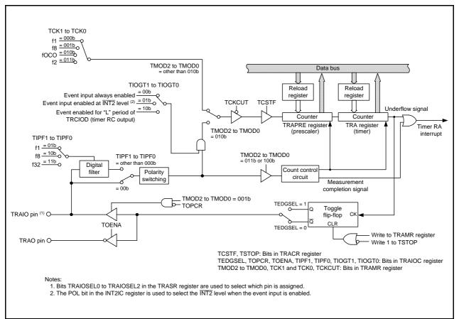
Figure 17.1 Timer RA Block Diagram
