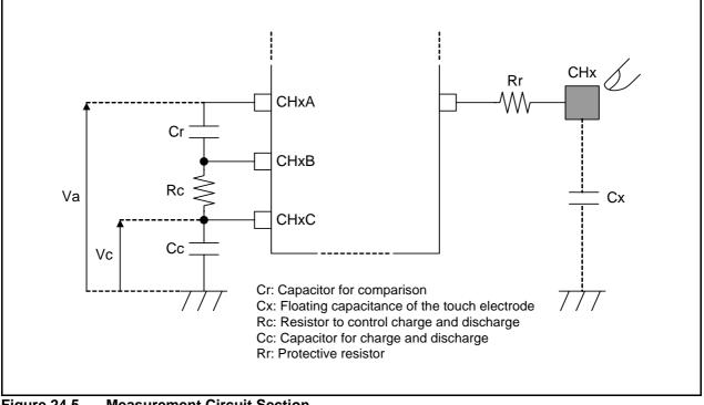
Figure 24.5 Measurement Circuit Section
