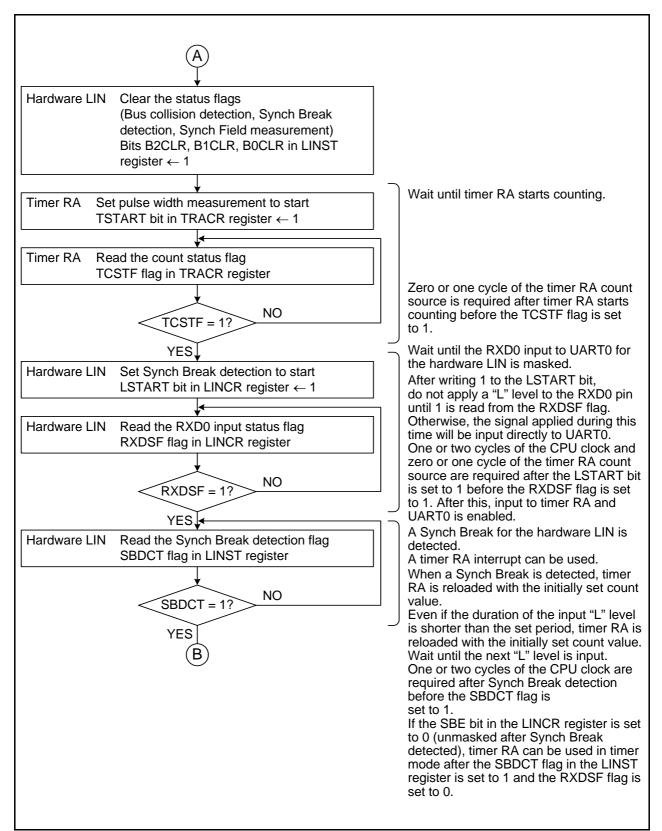
Figure 22.7 Header Field Reception Flowchart Example (2)
