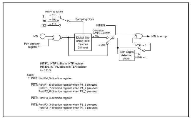
Figure 11.9 INTi Input Filter Configuration
