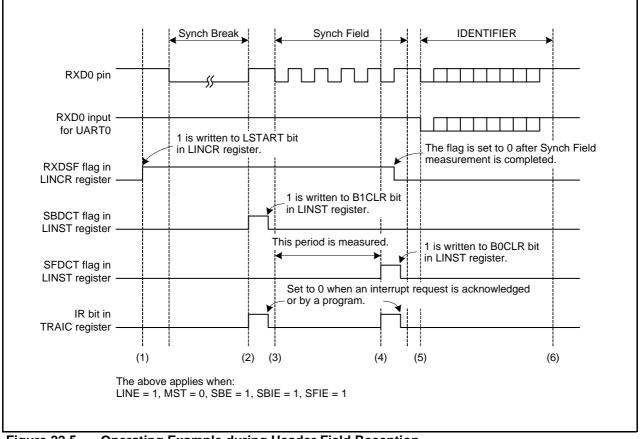
Figure 22.5 Operating Example during Header Field Reception
