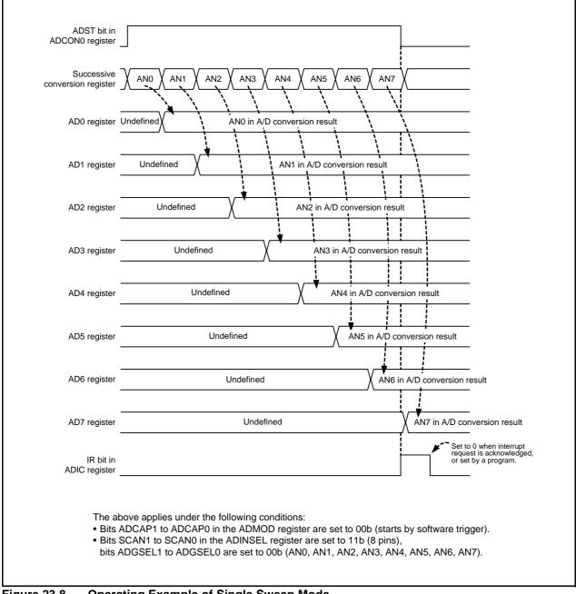
Figure 23.8 Operating Example of Single Sweep Mode
