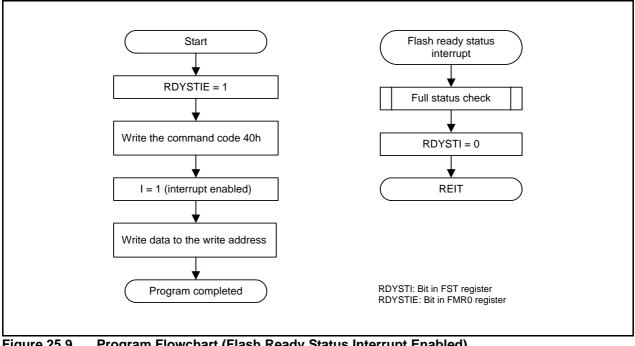
Figure 25.9 Program Flowchart (Flash Ready Status Interrupt Enabled)
