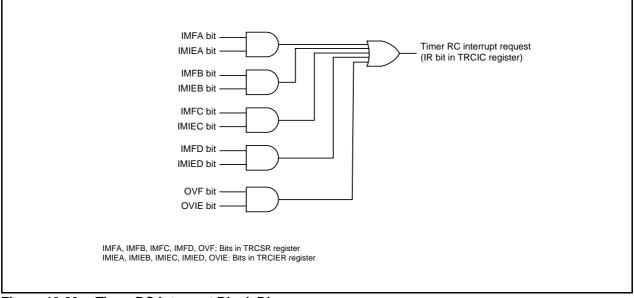
Figure 19.20 Timer RC Interrupt Block Diagram
