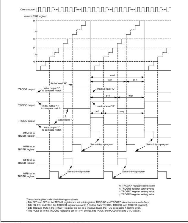
Figure 19.14 Operating Example of PWM Mode
