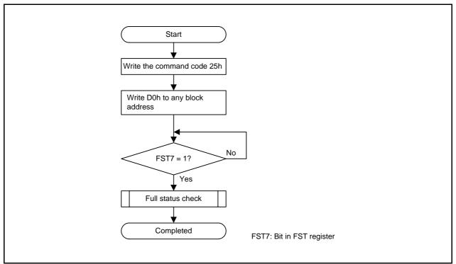
Figure 25.15 Block Blank Check Flowchart
