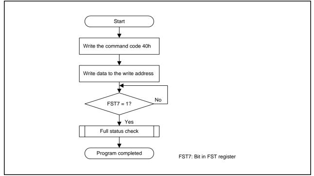
Figure 25.8 Program Flowchart (Flash Ready Status Interrupt Disabled)
