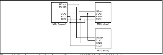
Figure 21.17 Communication Control Example (UART2) in Special Mode 2
