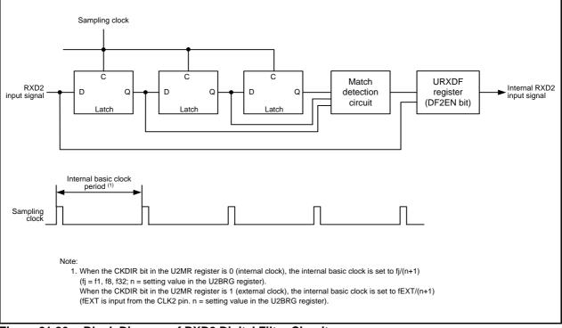
Figure 21.26 Block Diagram of RXD2 Digital Filter Circuit
