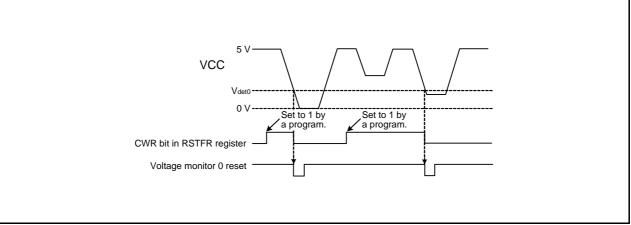
Figure 5.8 Operating Example of Cold Start-Up/Warm Start-Up Function
