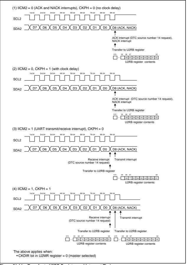
Figure 21.14 Transfer to U2RB Register and Interrupt Timing
