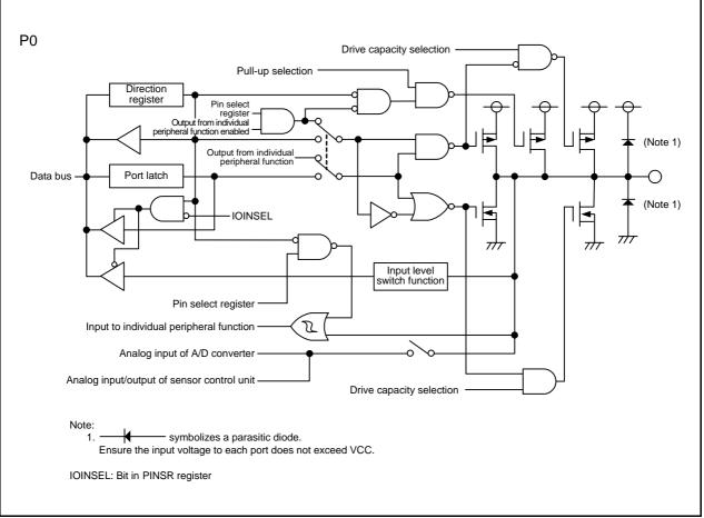
Figure 7.1Configuration of I/O Ports (1)
