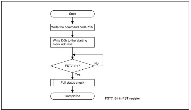
Figure 25.14 Read Lock Bit Status Flowchart
