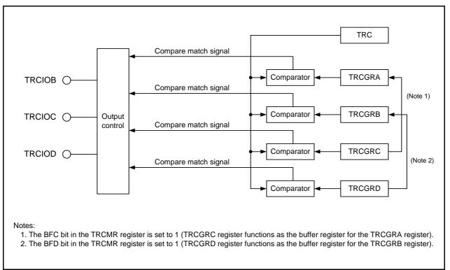
Figure 19.13 PWM Mode Block Diagram
