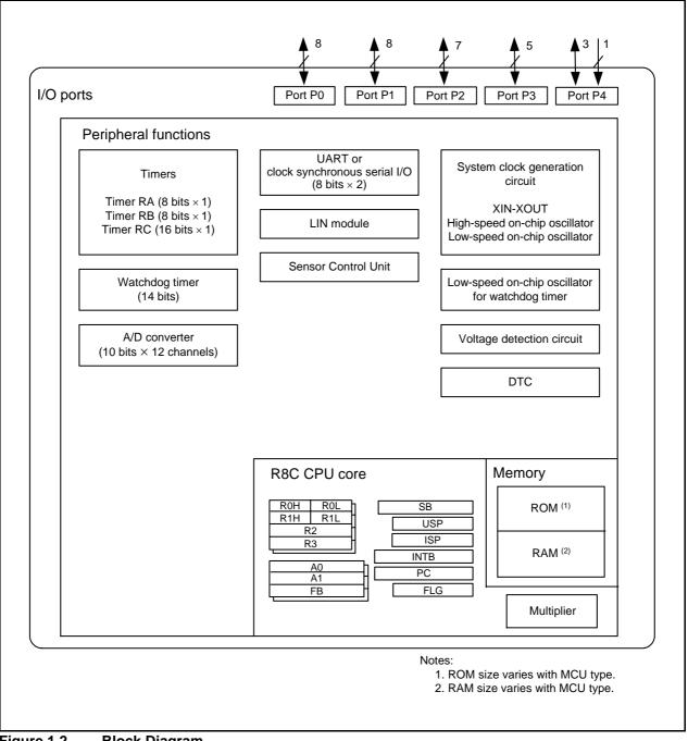
Figure 1.2 Block Diagram
