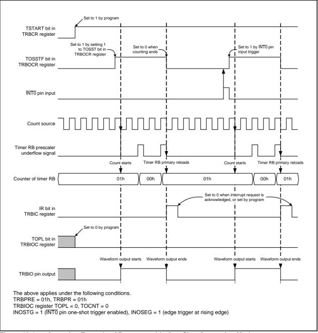
Figure 18.4 Operating Example of Programmable One-Shot Generation Mode
