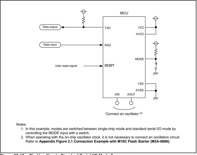
Figure 25.17 Pin Handling in Standard Serial I/O Mode 2
