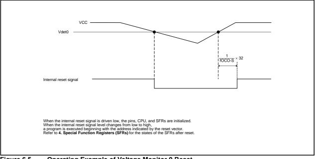
Figure 6.5 Operating Example of Voltage Monitor 0 Reset
