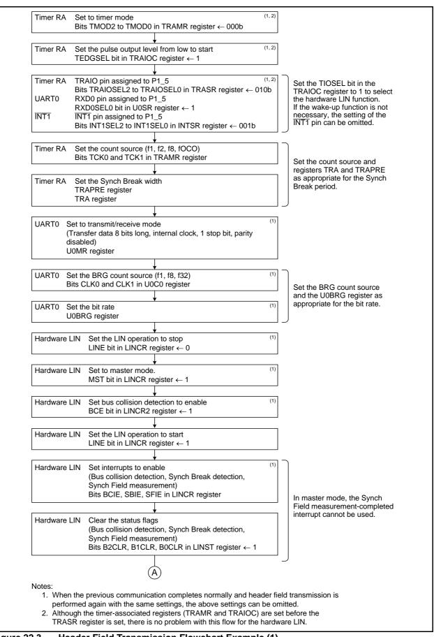
Figure 22.3 Header Field Transmission Flowchart Example (1)
