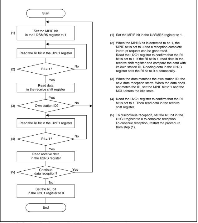
Figure 21.24 Sample Flowchart of Multiprocessor Data Reception
