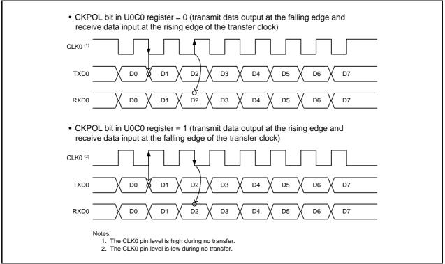
Figure 20.4 Transfer Clock Polarity
