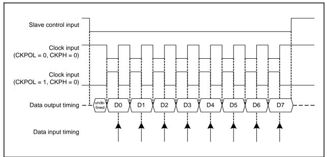
Figure 21.19 Transmit and Receive Timing (CKPH = 0) in Slave Mode (External Clock)
