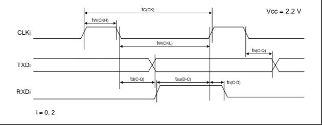
Figure 27.14 Serial Interface Timing Diagram when Vcc = 2.2 V
