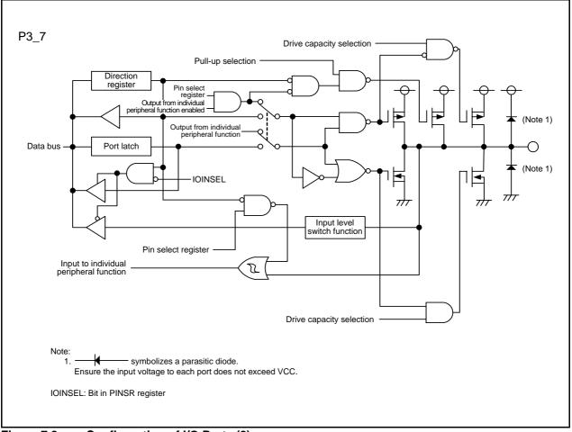
Figure 7.8 Configuration of I/O Ports (8)
