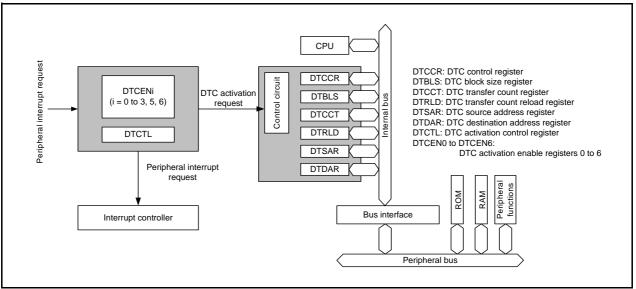
Figure 15.1 DTC Block Diagram
