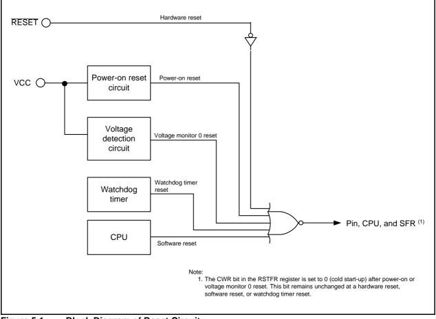
Figure 5.1 Block Diagram of Reset Circuit
