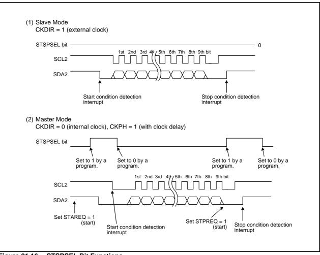
Figure 21.16 STSPSEL Bit Functions
