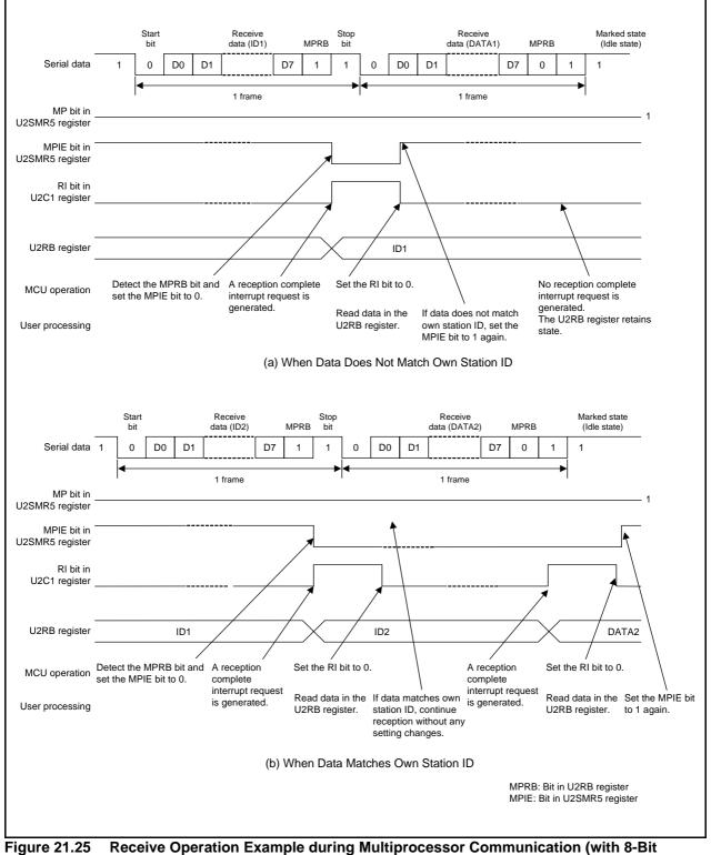
Data/Multiprocessor Bit/One-Stop Bit)
