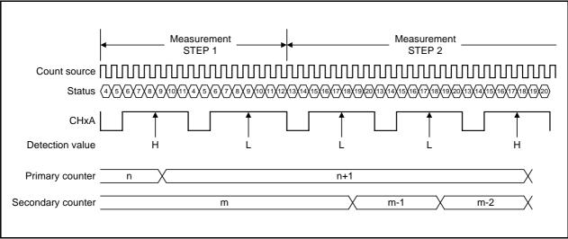
Figure 24.4 Detection Operation Example of Sensor Control Unit
