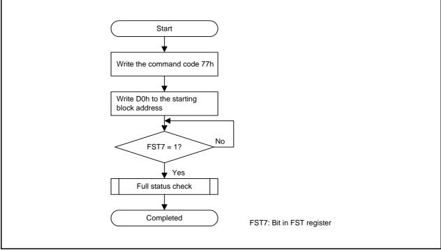
Figure 25.13 Lock Bit Program Flowchart
