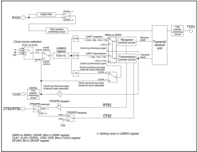
Figure 21.1 UART2 Block Diagram
