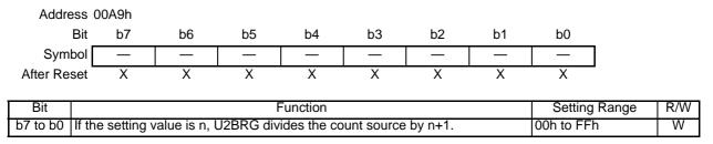
Write to the U2BRG register while transmission and reception stop. Use the MOV instruction to write to this register.
