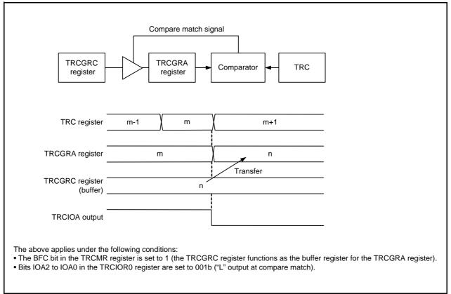
Figure 19.4 Buffer Operation for Output Compare Function
