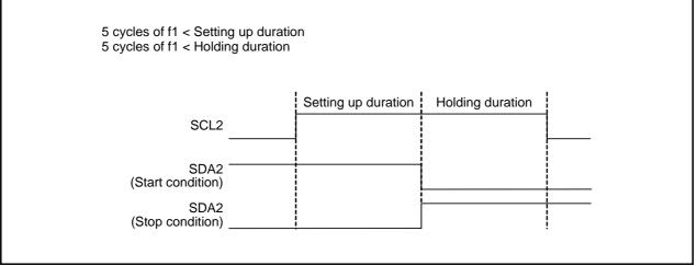
Figure 21.15 Detection of Start and Stop Conditions
