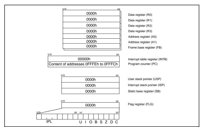
Figure 5.2 CPU Register Status after Reset
