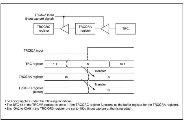
Figure 19.3 Buffer Operation for Input Capture Function
