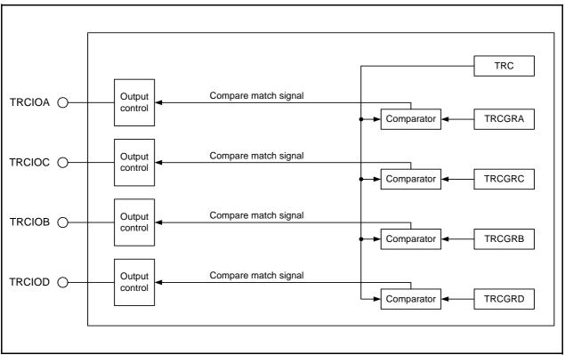
Figure 19.9 Block Diagram of Output Compare Function
