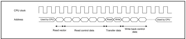
Figure 15.9 Example of DTC Operation Timings
