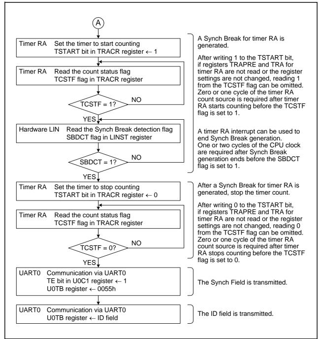
Figure 22.4 Header Field Transmission Flowchart Example (2)
