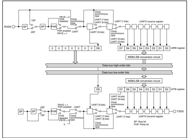
Figure 20.2 Block Diagram of UART0 Transmit/Receive Unit
