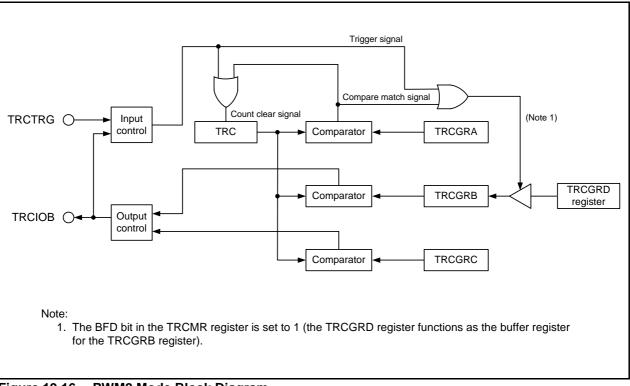
Figure 19.16 PWM2 Mode Block Diagram
