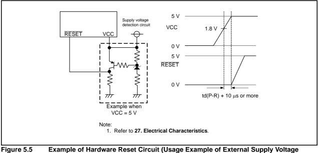
Figure 5.5 Example of Hardware Reset Circuit (Usage Example of External Supply Voltag Detection Circuit) and Operation
