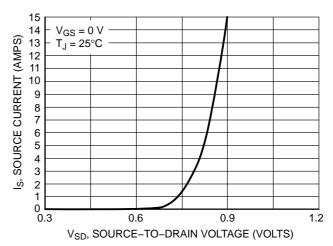
Figure 10. Diode Forward Voltage vs. Current
