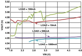
FIGURE 10. OUTPUT VOLTAGE vs INPUT VOLTAGE (MODE = HIGH, TA = +25°C)
