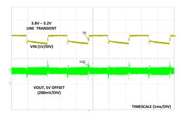
FIGURE 16. LINE TRANSIENT (VOUT = 5V)
