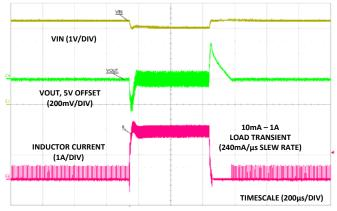
FIGURE 14. LOAD TRANSIENT (VIN = 3.0V, VOUT = 5V)
