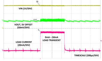
FIGURE 13. LOAD TRANSIENT (VIN = 3.0V, VOUT = 5V)
