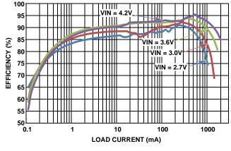
FIGURE 2. EFFICIENCY vs LOAD CURRENT (VOUT = 5V)
