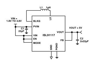
FIGURE 1. TYPICAL FIXED OUTPUT APPLICATION
