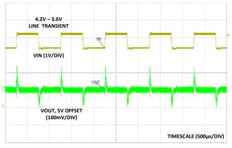
FIGURE 15. LINE TRANSIENT (VOUT = 5V)
