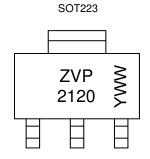
ZVP 2120 = Product Type Marking Code YWW = Date Code Marking Y or  $\overline{Y}$  = Last Digit of Year (ex: 5= 2015) WW or  $\overline{W}W$  = Week Code (01~53)
