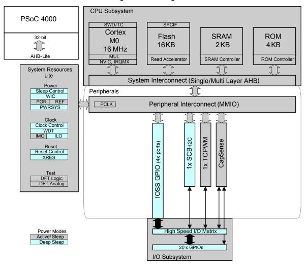
Figure 2. Block Diagram
